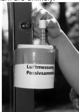
Mounting of NO 2 diffusive samplers
